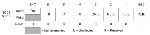
Figure 7. SCI control register 3 (SCC3)
