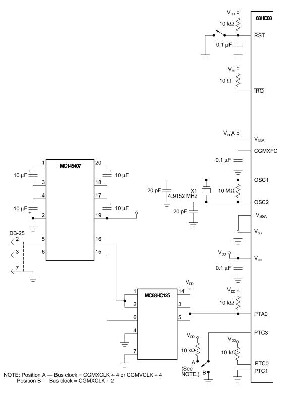
Figure 1. Monitor mode circuit
