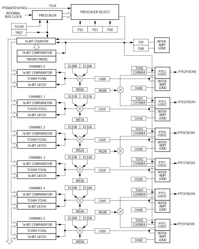
Figure 1. TIMA Block Diagram
