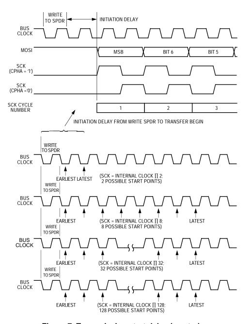
Figure 7. Transmission start delay (master)
