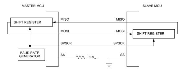
Figure 3. Full-duplex master-slave connections
