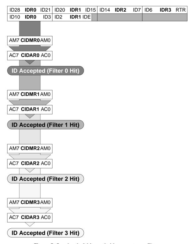
Figure 5. Quadruple 8-bit maskable acceptance filters
