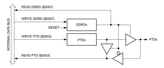
Figure 12. Port D I/O circuit
