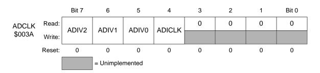
Figure 4. ADC clock register
