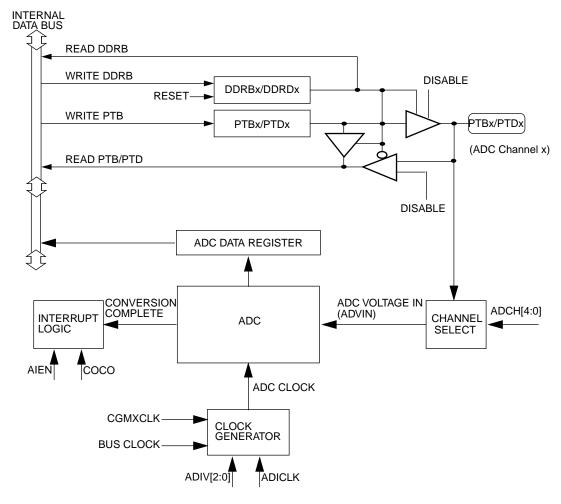
Figure 1. ADC block diagram
