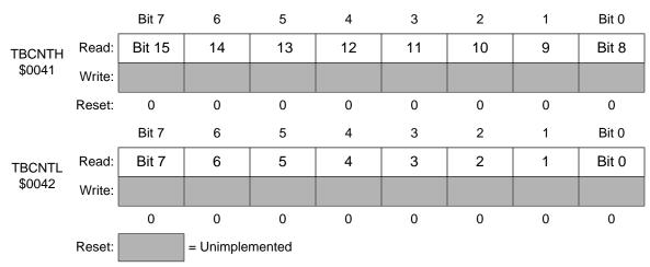
Figure 19. TIMB counter registers (TBCNTH:TBCNTL)
