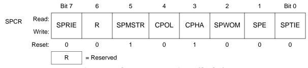
Figure 13. SPI control register (SPCR)
