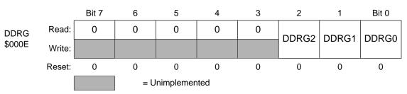
Figure 20. Data direction register G (DDRG)
