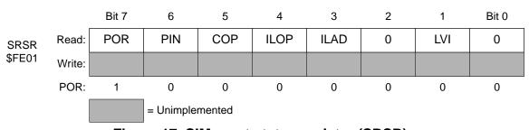
Figure 17. SIM reset status register (SRSR)
