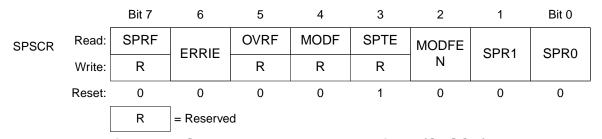
Figure 14. SPI status and control register (SPSCR)
