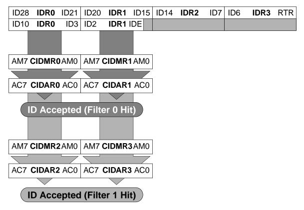
Figure 4. Dual 16-bit maskable acceptance filters
