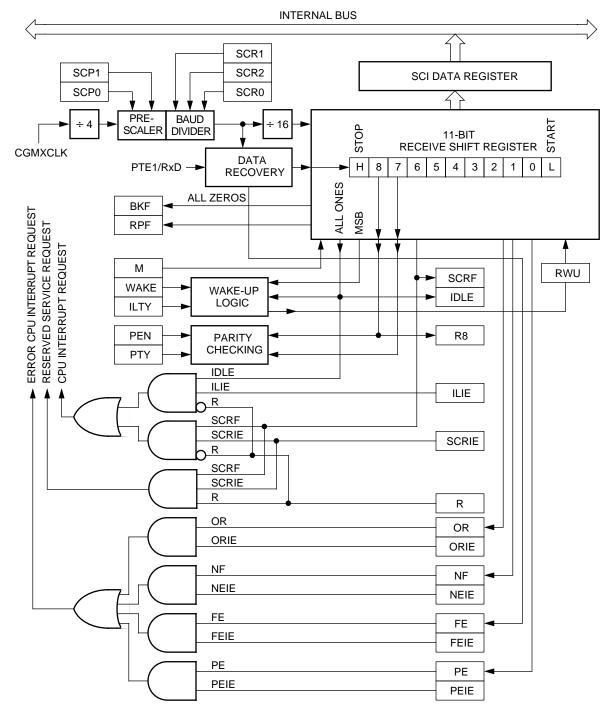
Figure 3. SCI receiver block diagram
