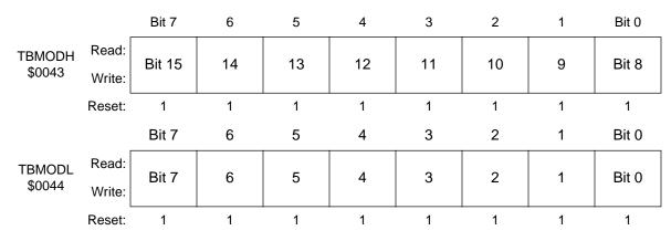
Figure 20. TIMB counter modulo registers (TBMODH:TBMODL)
