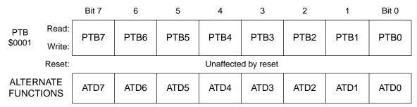
Figure 4. Port B data register (PTB)
