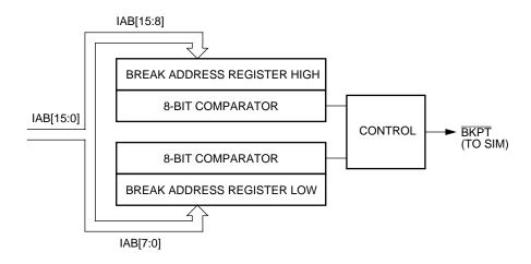
Figure 11. Break module block diagram
