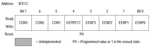
Figure 2. EEPROM Nonvolatile Register (EENVR)
