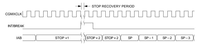
Figure 15. STOP mode recovery from interrupt
