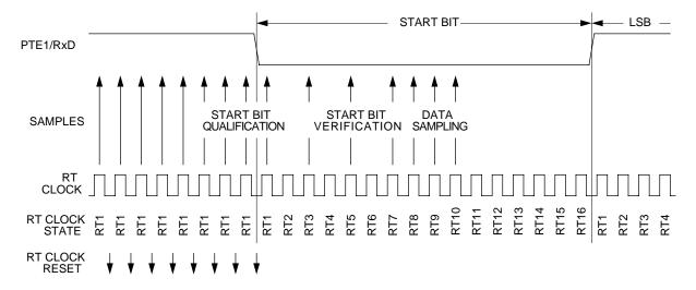
Figure 4. Receiver data sampling
