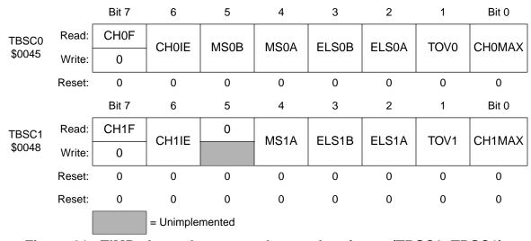
Figure 21. TIMB channel status and control registers (TBSC0-TBSC1)
