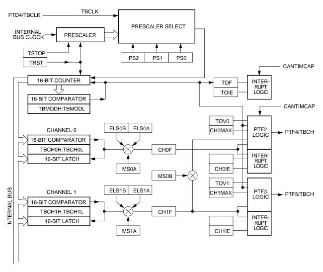
Figure 16. TIMB block diagram
