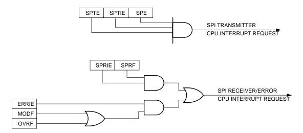
Figure 10. SPI interrupt request generation
