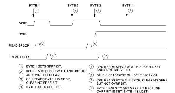
Figure 8. Missed read of overflow condition
