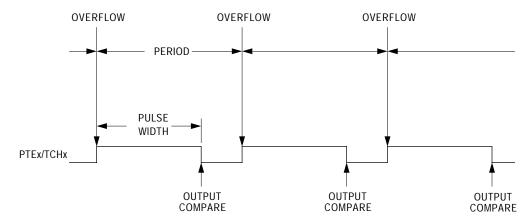
Figure 3. PWM Period and Pulse Width
