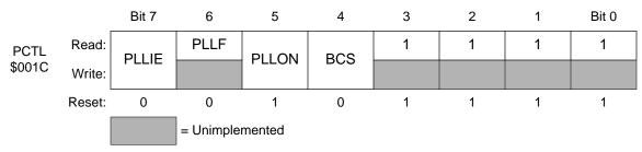
Figure 5. PLL control register (PCTL)
