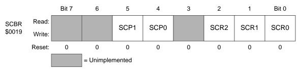
Figure 12. SCI Baud Rate Register (SCBR)
