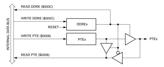
Figure 15. Port E I/O circuit
