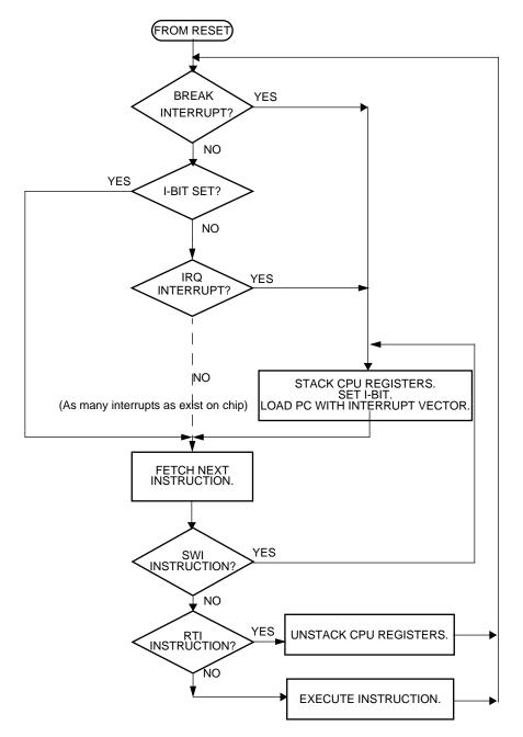
Figure 8. Interrupt processing
