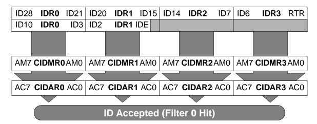
Figure 3. Single 32-bit maskable identifier acceptance filter
