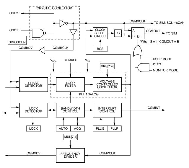
Figure 1. CGM block diagram
