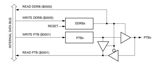
Figure 6. Port B I/O circuit
