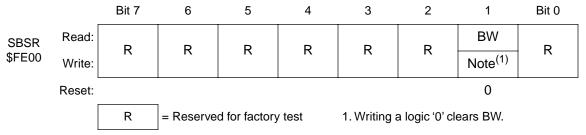
Figure 16. SIM break status register (SBSR)
