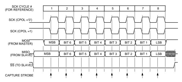
Figure 4. Transmission format (CPHA = '0')
