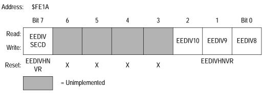
Figure 6. EEDIV Divider High Register (EEDIVH)
