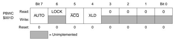
Figure 7. PLL bandwidth control register (PBWC)
