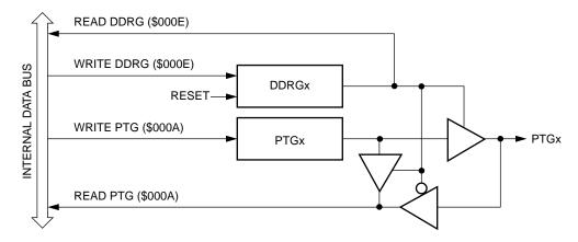
Figure 21. Port G I/O circuit
