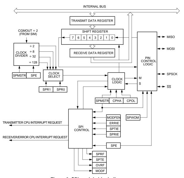
Figure 2. SPI module block diagram
