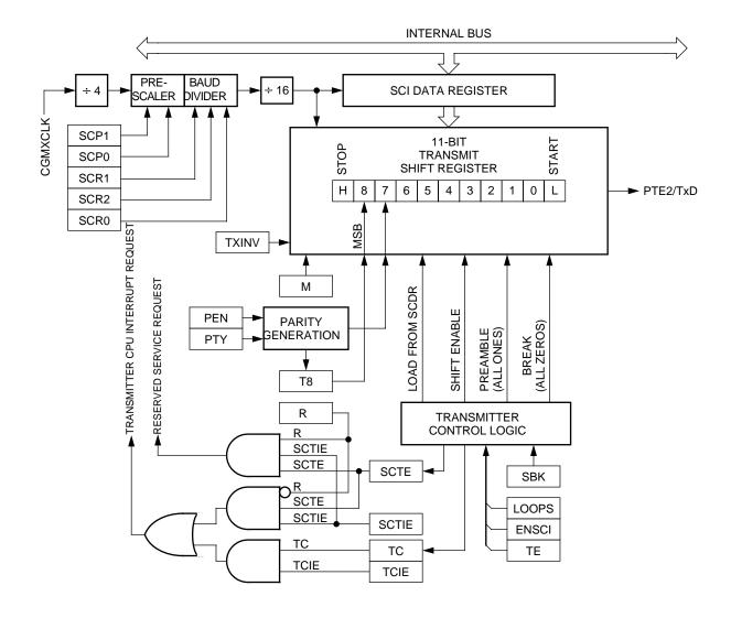
Figure 2. SCI transmitter
