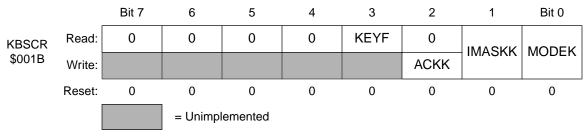
Figure 6. Keyboard status and control register (KBSCR)
