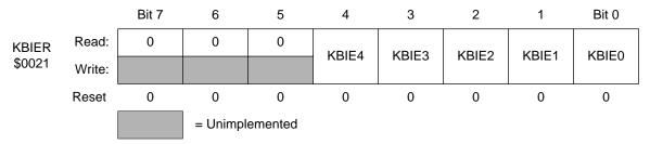
Figure 7. Keyboard interrupt enable register (KBIER)
