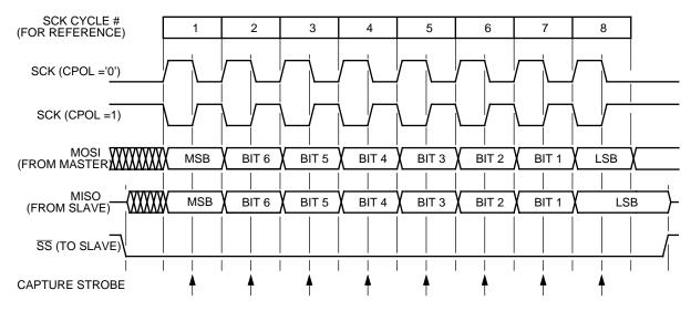
Figure 6. Transmission format (CPHA = '1')
