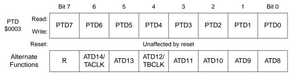
Figure 10. Port D data register (PTD)
