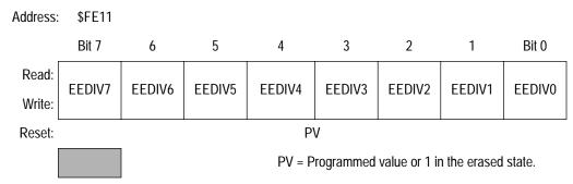
Figure 5. EEDIV Non-volatile Register (EEDIVLNVR)
