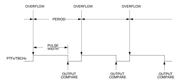
Figure 17. PWM period and pulse width
