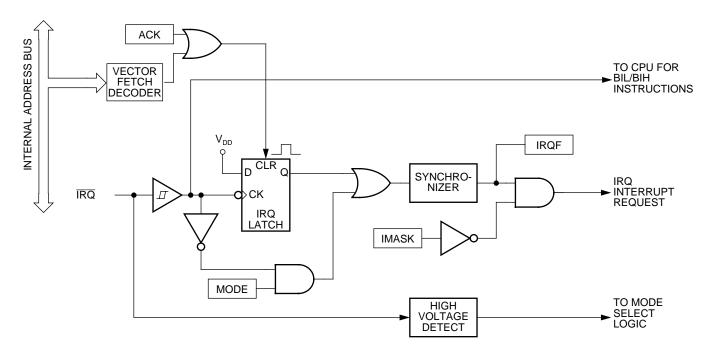
Figure 3. IRQ module block diagram
