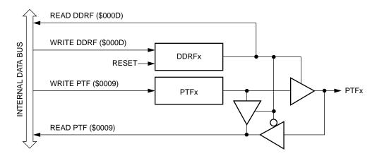
Figure 18. Port F I/O circuit
