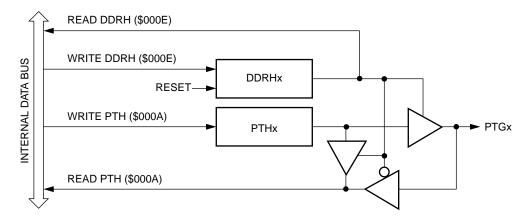
Figure 24. Port H I/O circuit
