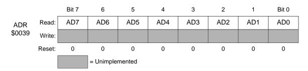
Figure 3. ADC data register
