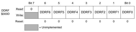
Figure 17. Data direction register F (DDRF)
