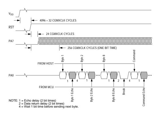
Figure 6. Monitor mode entry timing
