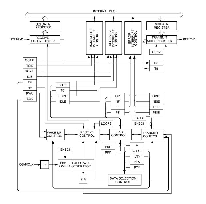
Figure 1. SCI module block diagram
