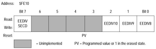
Figure 4. EEDIV Non-volatile Register (EEDIVHNVR)
