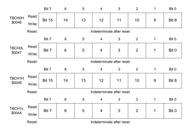
Figure 23. TIMB channel registers (TBCH0H/L-TBCH1H/L)
