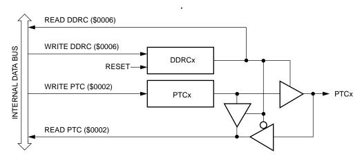
Figure 9. Port C I/O circuit
