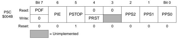
Figure 2. PIT Status and Control Register (TSC)
