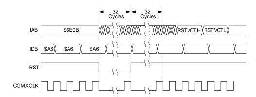
Figure 13. WAIT recovery from internal reset
