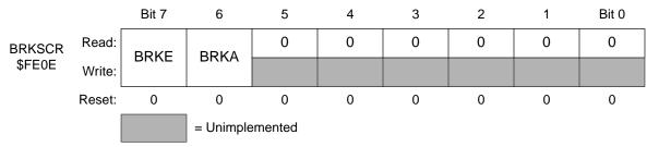
Figure 12. Break status and control register (BRKSCR)
