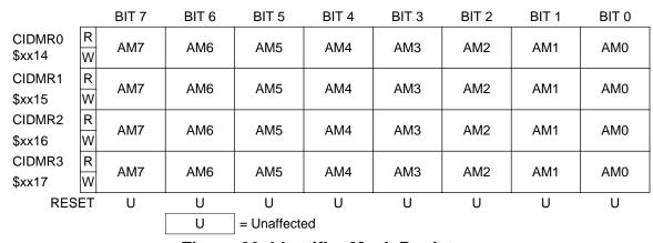
Figure 26. Identifier Mask Registers
