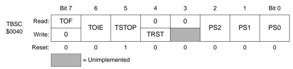
Figure 18. TIMB status and control register (TBSC)
