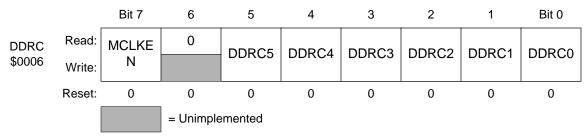
Figure 8. Data direction register C (DDRC)
