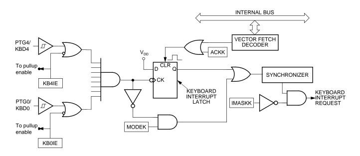
Figure 5. Keyboard module block diagram
