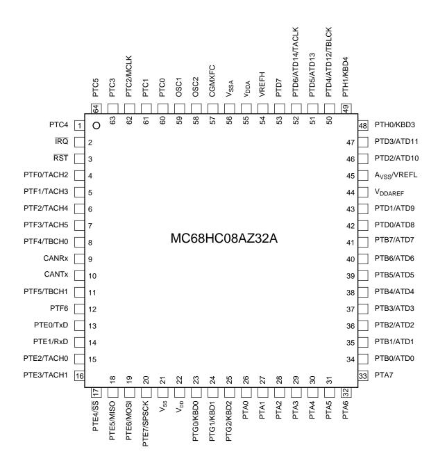
Figure 2. 64 QFP pin assignments
