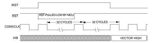
Figure 4. Internal reset timing
