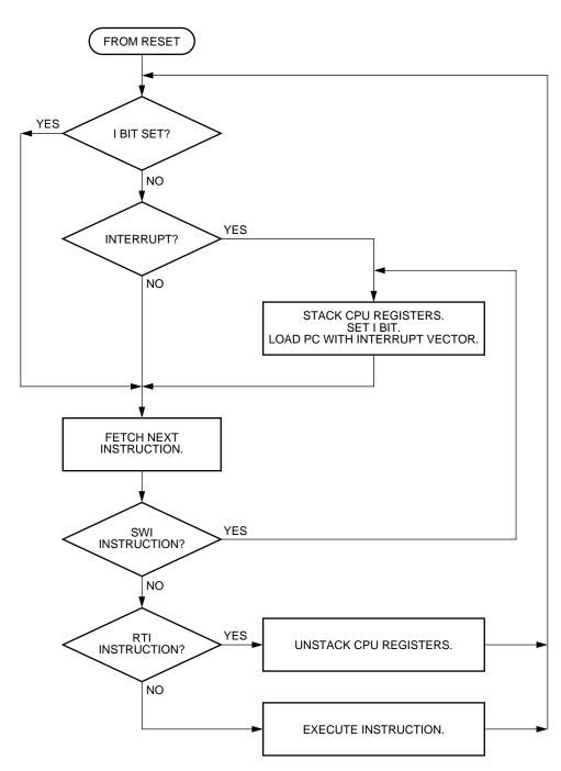
Figure 4. IRQ interrupt flowchart
