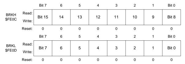
Figure 13. Break address registers (BRKH and BRKL)
