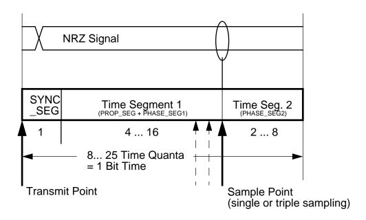
Figure 8. Segments within the bit time
