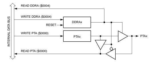
Figure 3. Port A I/O Circuit
